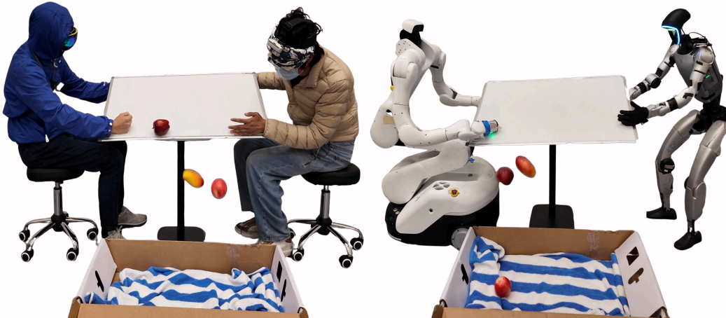
Figure 1: DUET . We introduce a dual-robot policy learning framework that features efficient learning from human demonstrations. Left: Two humans perform a collaborative manipulation task. Right: A heterogeneous dual-robot system mimics the human teachers.
