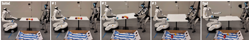
(T3: Board Tilting) G1 and Vega1 stand on the sides of a white board with three fruits on top ( Initial ). G1 and Vega1 approach the white board ( #1 ). G1 and Vega1 collaboratively tilt the white board ( #2 ). The fruits fall into the basket ( #3 ). G1 and Vega1 secure the board on the table with fruits in basket ( End ).
